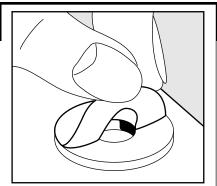
Remove the paper from both sides of the washer.
