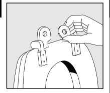
Attach washer to bottom of hinge.
